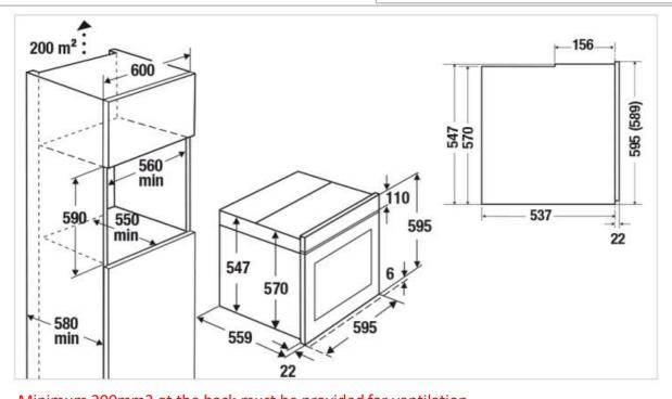
Minimum 200mm2 at the back must be provided for ventilation.
